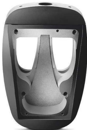
LEFT: Monoblock tweeter moulding seen from above. The horn section (empty here) is filled with foam to absorb the rear radiation from the tweeter dome, pictured above. Voids maximise the internal volume available to the bass driver
