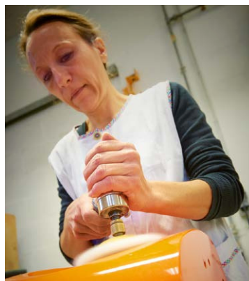
◀ The cabinets for Focal's Utopia, Sopra, and Electra Series speakers are all assembled in France, seen here being sanded, painted, and polished. Then finally, drivers are inserted.
